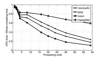
Figure 4: Efficiency ratio for an exploration of 1000 configurations with an exponentially growing number of processors.
