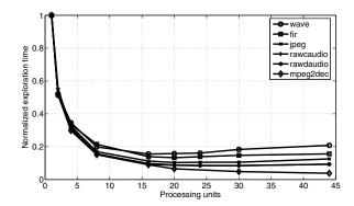
Figure 2: Normalized time required for an exploration of 1000 configurations with an exponentially growing number of processors.
